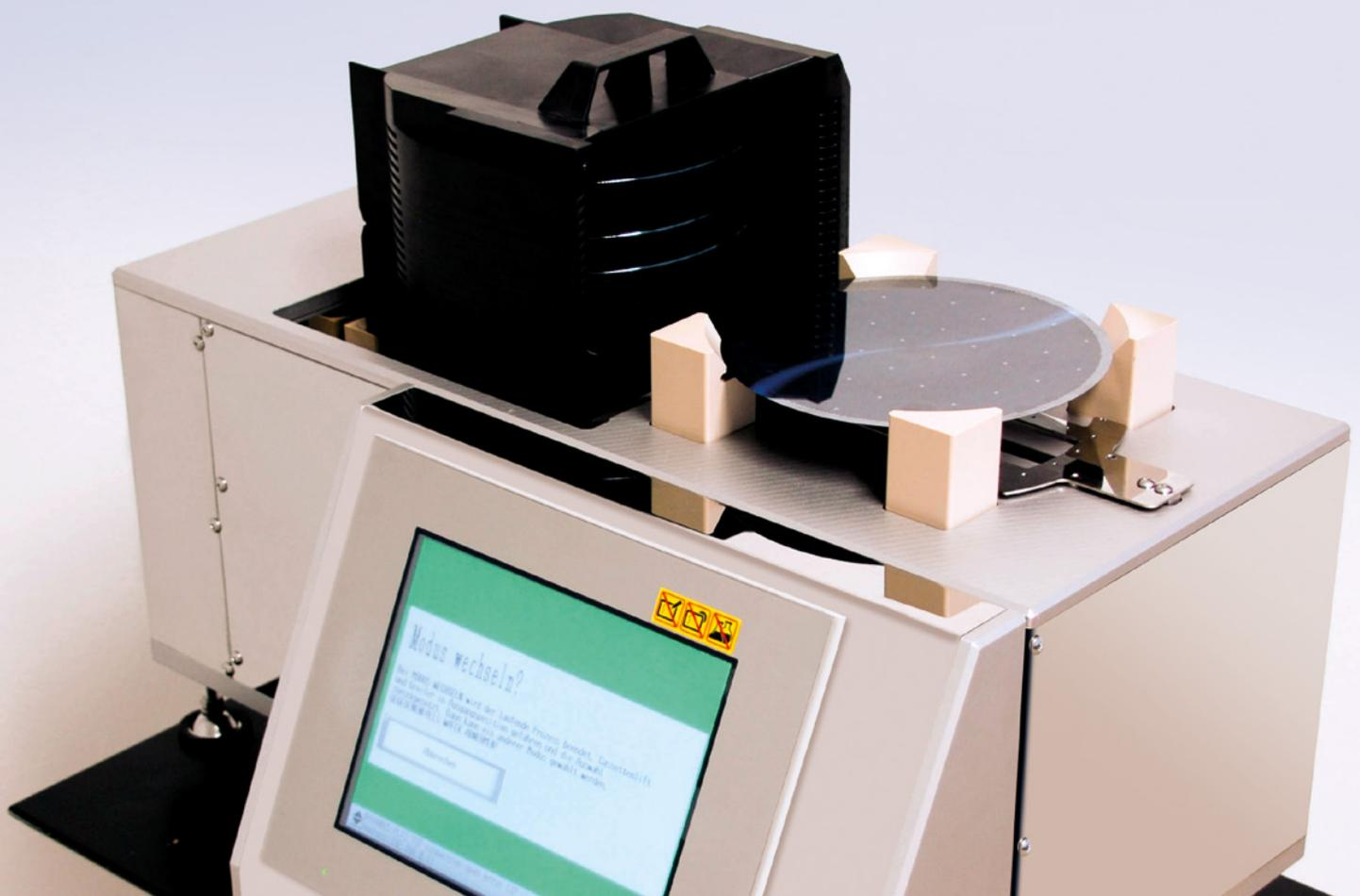
Machine for semi-automatic loading and unloading of 100mm (4"), 160mm (6") and 200mm (8") from a cassette. Vacuum or vacuumless grabber.
